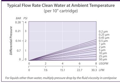
The micron ratings shown at various efficiency and beta ratio value levels were determined through laboratory testing, and can be used as a guide for selecting cartridges and estimating their performance. Under actual field conditions, results may vary somewhat from the values shown due to the variability of filtration parameters.
